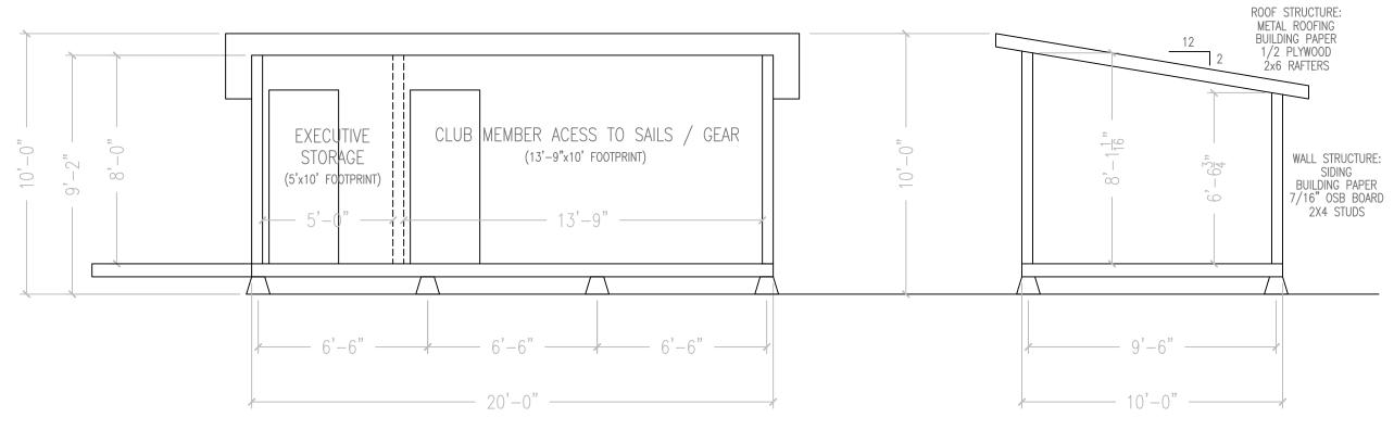
TO BE BUILT ON A STEEL FRAME WITH TRAILER HITCH AND LEAF SPRING ATTACHMENTS WELDED ON FOR FUTURE MOVING PURPOSES IF NECESSARY.
